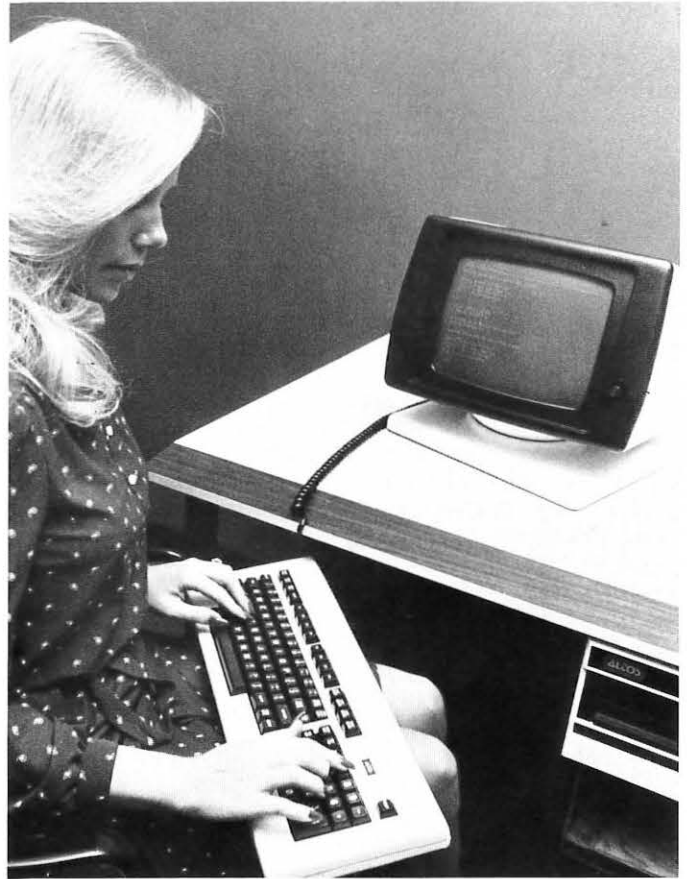
This Altos 1 user-friendly "smart" terminal is said to increase operator productivity by enhancing system performance. It features rotatable-tiltable screen, easy-to-read phosphor display to reduce eyestrain, and detached keyboard with 6-foot cable.
