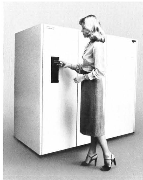
Masstor Systems Corporation, Sunnyvale, CA, now offers a tape cartridge-based system that gives users a data storage capacity of 55 billion bytes per unit. It gives users over five times the storage capacity of IBM's 3850 mass storage unit. Access to the tape cartridges is through an access panel in front of the unit.
